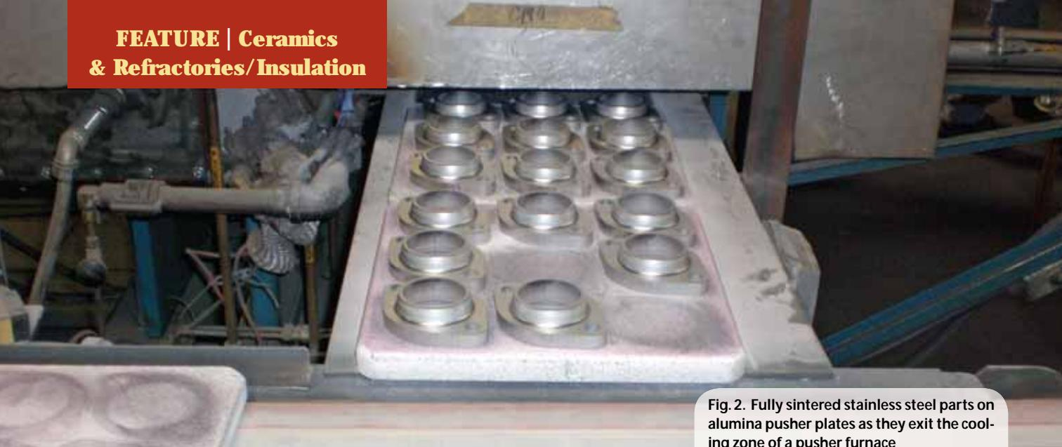
**Fig. 2. Fully sintered stainless steel parts on alumina pusher plates as they exit the cooling zone of a pusher furnace**
